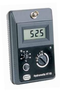
The HT 65 unit is an electronic wood moisture meter that uses the resistance principle of measurement for precisely measuring sawn timber (up to 180 mm in thickness), chipboards, veneers, wood chips, and similar bulk materials. The unit is used for individual measurements before and after processing.
